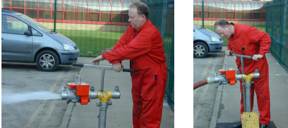
Fig. 4.1 Testing an underground hydrant using a standpipe. Photographs courtesy of Essex County Fire and Rescue Service.
