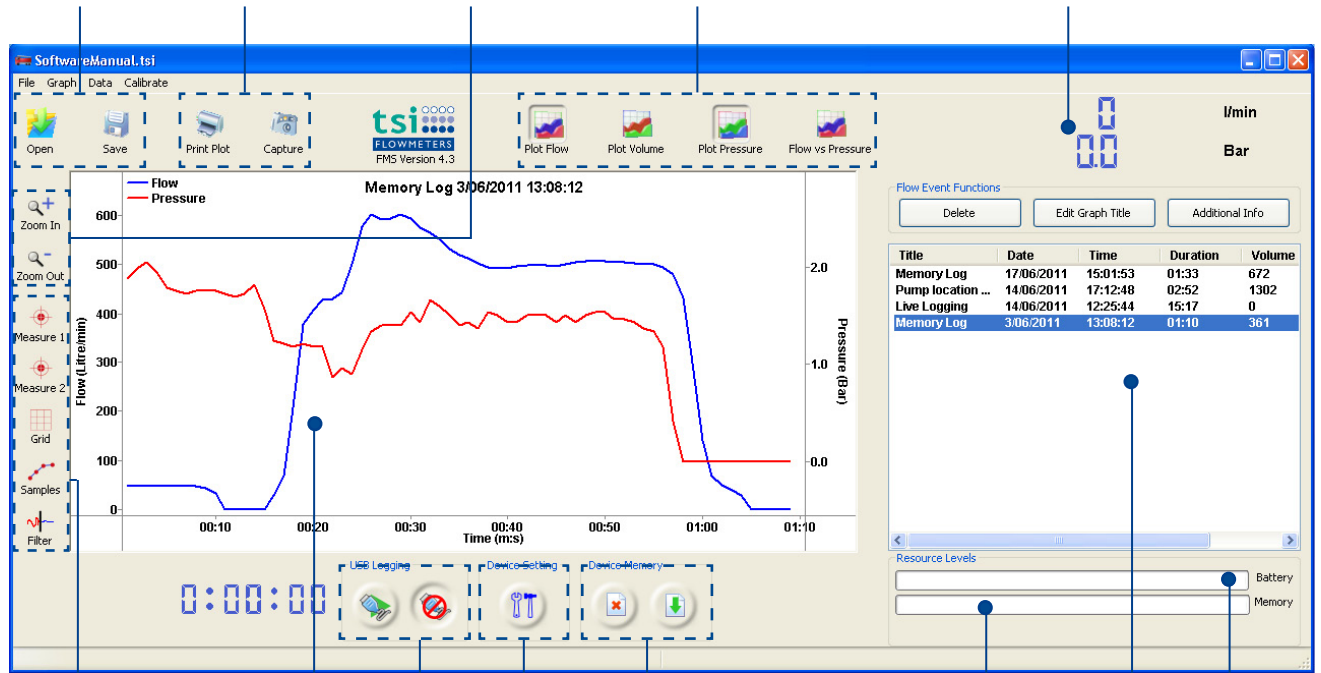
Plot Data Flow / Volume & Device Visualisation Pressure Plotting Area Setting USB Logging Data Upload from Logger Log Files Logger Memory Battery Level Availability Indicator
