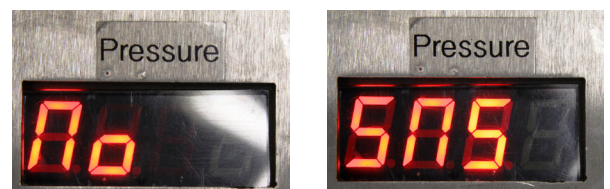
Fig. 5.3 This is how No SNS (flow sensor not connected) is displayed on the LED readout
