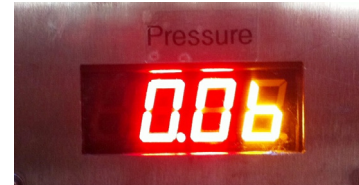
Fig. 3.5 After 3 seconds, LED readout displays pressure in bar
