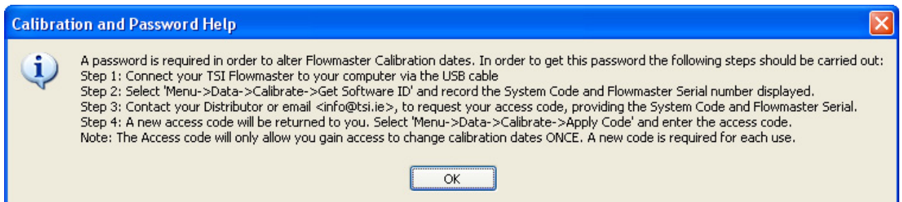
Fig. 5.9 The calibration password help menu is accessed by selecting the 'calibrate access help' tab from the calibrate menu
