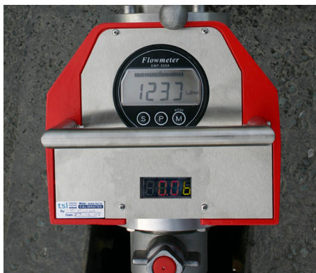
Fig. 4.2 An example of a flow readout and a residual pressure reading. Photograph courtesy of Laois Fire Service.
