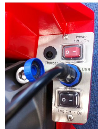
Fig. 4.9 Flowmaster control panel
