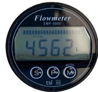
Fig. 1.7 Use totalise function of Flowmaster to record volume released during flushing for input to leakage figure records
