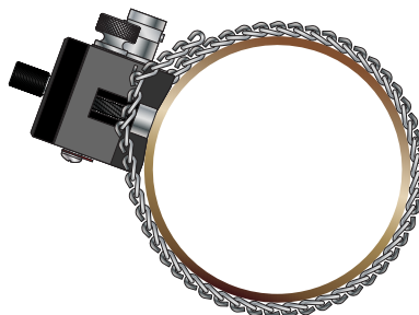
Figure 29: DTTSU transducers mounted
