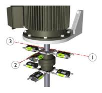
Place yourself at the position corresponding to the second measurement position, where it is easiest to turn the shafts through 180°.
