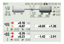
The screen displays measurement results, dimensions, target values if any, file name, date and time, serial number of the display unit, program, program version, calibration date and tolerances.
