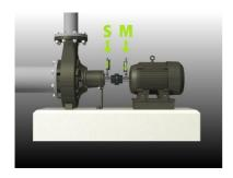
After rotating the shafts into different measuring positions the system calculates the relative distance between the two shafts in two planes. The distances between the two measuring planes, distance to the coupling and distances to the machine feet are entered into the system. The display box then shows the actual alignment condition together with the position of the feet.
