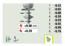
Adjust the angular error by placing shims under the bolts as required (negative bolt value means that shims should be added.) The angular error is displayed live in the first direction when the sensors are placed in position number 1, and in the second direction when they are placed in position number 2.
