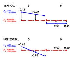
After having entered these feet values, the system calculates how the movable machine should be positioned (target position) in cold condition in order to obtain perfect alignment during running condition.
