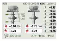
The screen displays measurement results, dimensions, file name, date and time, serial number of the display unit, program, program version, calibration date and tolerances.
