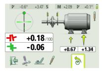
Rotate the shafts to the 12 or 6 o'clock position to make adjustments in the vertical direction. The angle guide helps you to reach the right position.
