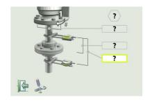
Set the sensors at approximately the same rotational angle at the first measurement position, with bolt number 1 to the right.
