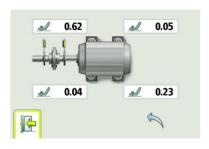
Make the necessary corrections and then check each foot again (the values show approximately how many shims that are needed to eliminate the soft foot).
