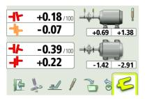
The Measurement Result screen shows coupling values and foot values in both the vertical and horizontal direction.
