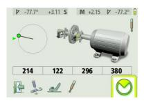
Set the sensors so that they are approximately at the same rotational angle at the first measurement position.
