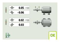
In the example above, the movable machine should be vertically adjusted to a position with an angular misalignment of +0.05 mm/100 mm and an offset of -0.06 mm.
