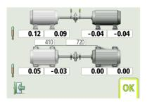
In the example above, the stationary machine will shrink vertically by 0.12 mm at the rear feet and 0.09 mm at front feet while the movable machine will expand 0.04 mm while running.
