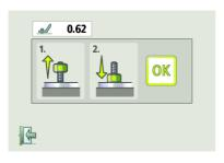
Loosen the bolt fully and then tighten it firmly, preferably with a dynamometric wrench.
