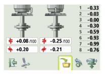
The Measurement Result screen shows coupling values in both directions, and bolt values.
